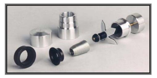
**Explanation:** The reason for this is quite simple, a counterclockwise rotation of the spring forces the coils to become smaller beause you are in fact rotating it in the direction of its windings. Trying to rotate the spring clockwise will work against the windings and this will make the spring become bigger thus making it more difficult or possibly impossible to move freely in its holder.
