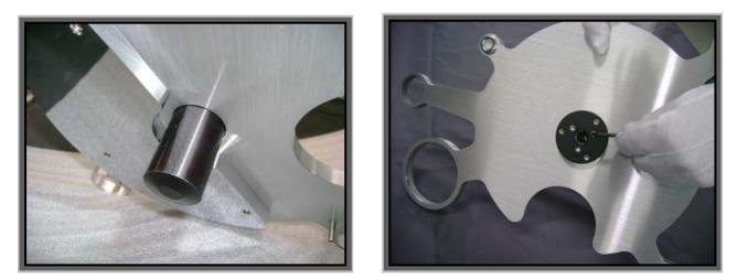
Assembling the spindle holder to the sub-chassis
