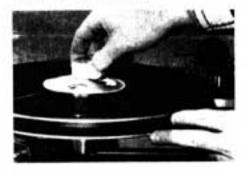
The action of the coupling disc and the tapered washer creates a vacuum under the record for better coupling of the playing surface to the turntable. You will notice that it also flattens out most warps.
