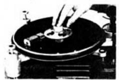
4) When you are satisfied that you have found the best weight arrangement for your turntable, make a note of the exact position you have chosen (i.e., the large weight placed at 7 o'clock with the inside edge 1.5" from the center spindle. Locate the carrier rod and slide the weight(s) you have chosen into the rod over the threaded end.
