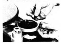
We suggest that you do not completely tighten either the arm board or the tonearm at this time. Tighten partially, allowing for whatever fine adjustments may be necessary. Rotating the arm board in either direction will help you fine-tune this tonearm / cartridge lateral tracking geometry. When you are satisfied that the tonearm is adjusted properly, TIGHTEN ALL CLAMP SCREWS AND ARM HARDWARE SECURELY!
