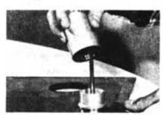
Locate the appropriate hex key and remove the top screw which holds the levelling knob in place. (This is the large black screw directly on top of the suspension tower assembly.)
