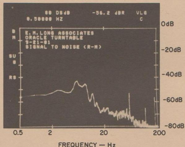
**Fig. 9B**—Similar to 8B but with the Rumpel-messkoppler. The arm resonance is still evident, but the spike at 20 Hz is not, indicating it is probably an artifact of the test disc.
