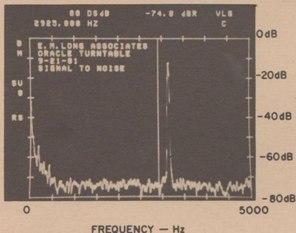
**Fig. 8A**—Spectrum of signal-to-noise ratio with B&K 2010 test disc. (Note: Scale is linear.)
