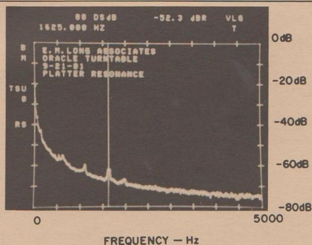
**Fig. 10—Spectrum of a platter resonance.**
