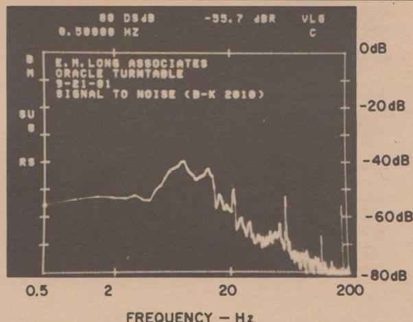
**Fig. 8B**—As in Fig. 8A but the increase from 7 to 10 Hz, but the level is over 40 dB down from the 10 cm/S reference. Tonearm resonance is responsible for most of
