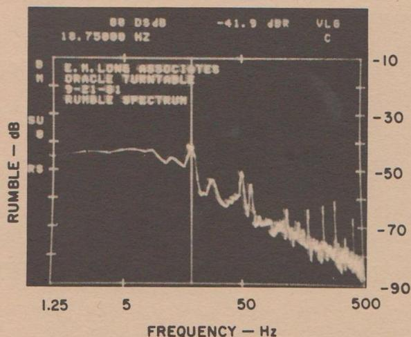
**Fig. 4—Rumble spectrum, with most components below 20 Hz. Spikes are harmonics of hum and occur below -60 dB.** Resolution of spectral detail is excellent. (Note: Unless noted, 0 dB ref. is 10 cm/S lateral groove modulation.)
