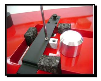
Note: The suspension is blocked with foam pieces and two aluminum blocks jamming the floating chassis against the main plinth. The small foam pieces are designed to keep the inner chassis from moving sideways. It is important to use them if you have to transport or ship your Paris turntable.
