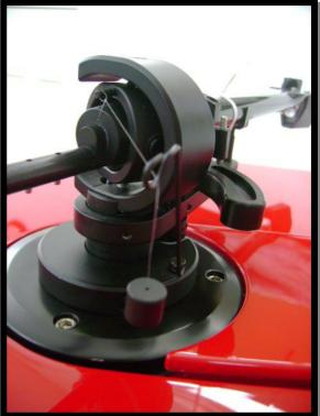
The Azimuth is done by viewing the phono cartridge from the front of the turntable. It is done by making sure the stylus tip is sitting perfectly vertically in the record groove. For the Paris tonearm, the whole arm tube can be rotated by loosening the socket head set screw at the rear of the tonearm.
