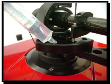
Important note: Do not make this adjustment with the stylus resting on the record! Place the tonearm in the arm rest and hold it while doing this adjustment to prevent damaging the stylus of your phono cartridge.
