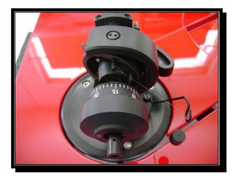
The anti-skate weight will attach near the gimbal bearings on the stem above the tracking force counter weight at the rear of the tonearm. Guide the nylon string in the eyelet of the metal wire support at the rear left side of the tonearm.
