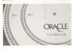
Note 3: The use of incandescent or fluorescent lighting is required to read the calibrator disc.
