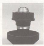
Note 4: Before installing the spring back into the module, pull on the spring at the wider end to stretch it as this will cause it to seat well in the thread.
