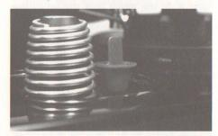
Note 3: With the spring adjusted as per step 2, the lip of the gauge should be well above the surface of the plinth. If the lip is below, it is an indication that the spring used is not suited for this tone arm application, it is too weak. Identify the color code and use the next stiffer spring. With a new spring start the procedure from step one.
