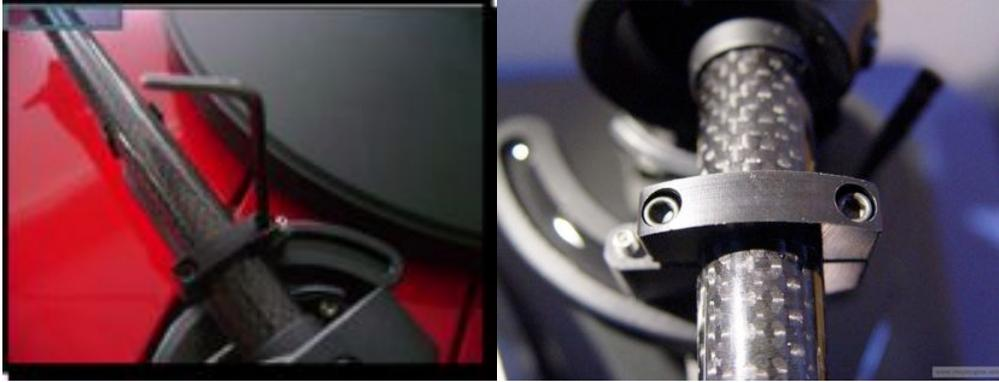
1. The center of the clamp mounted on the tone arm tube is at exactly 194,88mm (7,675") from the front edge of the tone arm tube.
