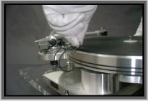
**Note:** Remember that each time the platter is removed from the spindle holder a certain quantity of oil will be lost ... the oil syringe we supply contains 4cc of oil. The special mix of Synthetic / PTFE lubricating oil supplied with your Delphi Mk VI is designed to protect and preserve the mating parts for many years. Unless contaminated
