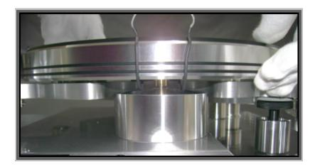
Rotate the platter by hand just so the installation tool is out of the axis on the motor and the drive belt starts engaging in the motor pulley.
