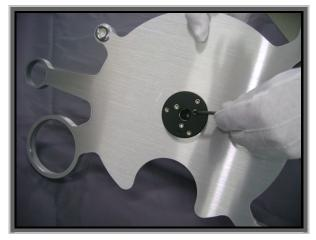
Assembling the spindle holder to the sub-chassis
