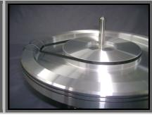
**Explanation** ... If the drive belt remains at the bottom of the platter around the inner hub there will be a misalignment with the height of the motor pulley. When the platter starts rotating the drive belt will then jump out of the motor pulley.
