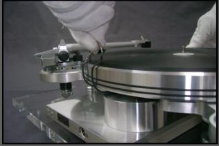
• Flip the drive belt installation tool towards the center of the platter as indicated in the picture below.
